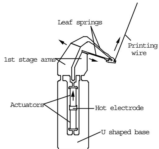
**Fig. 6:** Two-staged Differential Motion Mechanical Amplifier
